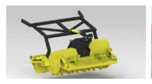
**Hydraulic front plate** makes perfect material flow to the up-cut rotor. Hydraulic push bar and rear roller are used for pushing down trees and bushes.
