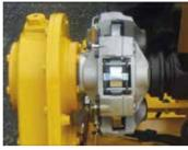
**POC clutch** protects the transmission line all the way through
