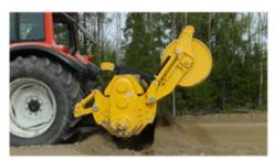
**Hydraulic front plate** and rear roller. Suokone made side gearbox is designed for heavy use and easy maintenance.
