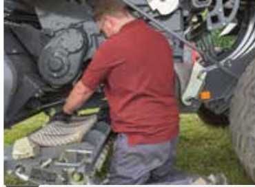
Ample accessibility offering straightforward knife removal
