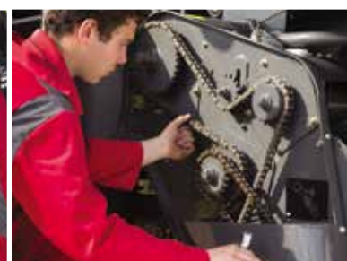
4. Checking the pick-up chain tensions.
