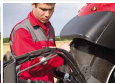
6. Greasing the PTO shaft.
