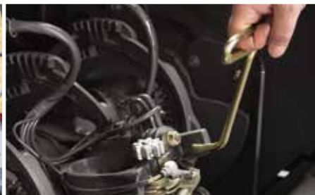
Each knoter head can easily be lifted for inspection and service.
