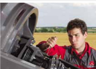
5. Adjusting the flywheel slip clutch.
