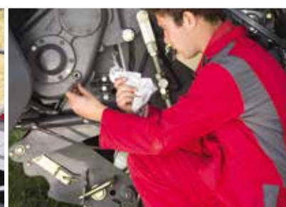
3. Checking the cutter gearbox oil level.
