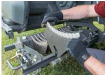
Ample accessibility offering straightforward knife removal
