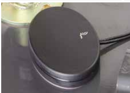
AGCOMMAND combined GPS & GSM antenna.
