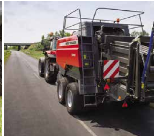
The tandem axle allows for high road speed and gives superb ride comfort between fields.
