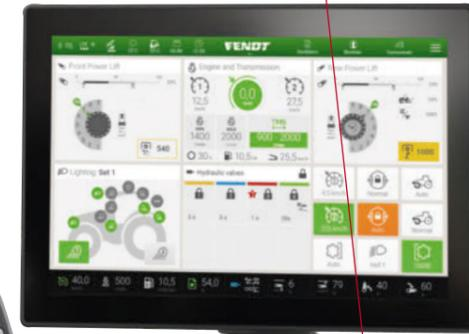
Use the central pushdial to decide what to display on the Fendt 300 Vario. This includes four quick access keys for Back, Launchpad, Overview, Individual Operation Manager (IOM) and switching between terminal and dashboard.
