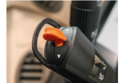
Limiting the tilt angle for safety: on the Fendt CargoProfi, you can limit the tilt angle when loading very high trailers. The Memo function is especially practical for repeating sequences, for example, the horizontal lower position can be targeted automatically. The weighing function gives you more control over the load weight.
