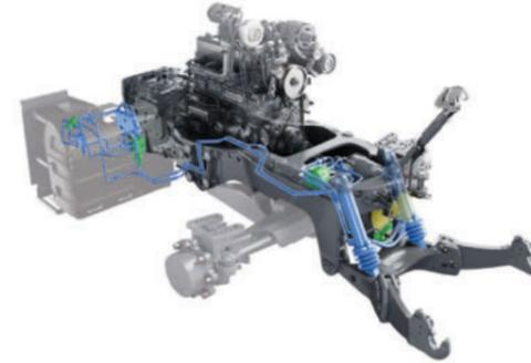
The front power lift is fully integrated and sits tight against the vehicle. This keeps the linked machines highly manoeuvrable. The lower links have a particularly good bottom grip and can be folded for parking. Bellows protect the lifting cylinders against stone impact. The vibration damping fitted as standard prevents bounce and guarantees safe driving and comfort.
