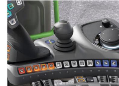
With the orange reverse lever, the driver can easily change directions with their left hand. Hold the lever down and the Vario stops. Release the lever and the tractor automatically drives in the preset direction.
