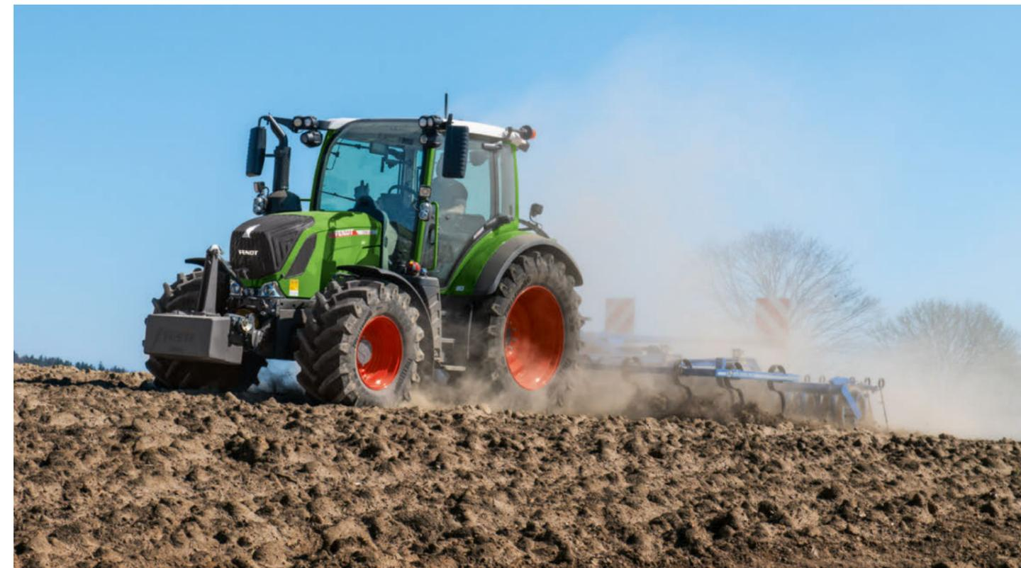
The smart power-boost concept Fendt DynamicPerformance (DP) on the Fendt 314 Vario releases up to 10 hp more power on demand. This is regulated depending on the operating conditions at any speed. You can also benefit from PTO power either at a standstill, for soil cultivation or during transport. The benefit is a lightweight tractor with more power and less fuel consumption per hectare.
