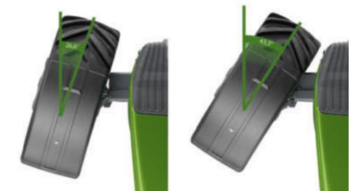
At the headland or during front loading work, you benefit from VarioActive steering\* as you can already reach full wheel impact with just one steering wheel rotation. Up to 8 km/h the superimposed steering system is unrestricted, from 8 to 18km/h the superimposition effect is linear.
