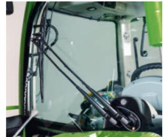
The clever ventilation and air-con design distributes the air perfectly from the steering column and from a side vent for the right window. There is also an overpressure and auto defrost function. The inside temperature is displayed on the dashboard. The foldable roof hatch provides draught-free ventilation.
