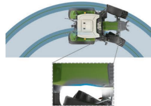
**Self-levelling front axle suspension for greater area coverage and traction**
