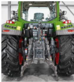
**Hydraulics system with up to 110 litres of flow volume**
