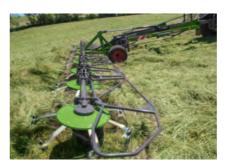
The large, forward-running transport wheels make sure it runs very quietly with a consistent working depth.
