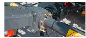
The overload protection on the main drive joint shaft increases operational reliability and makes the Lotus tedder drive train exceptional durable.
