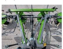
The three-point tower with three-material bearing bushings in the folding hinges is both durable and particularly maintenance-friendly.
