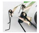
Because the wheel is close to the tines, the machine adapts beautifully to the ground, every
