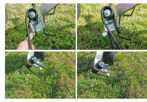
A simple adjustment of the tines on the outer rotor activates the edgeprocessing mechanism. This puts the tines in the innermost position for a neat field edge and to perfectly distribute the mowed crop.
