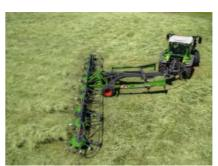
You can set the working depth to any level. With the help of the easily accessible crank, you can accurately adjust the raking height.
