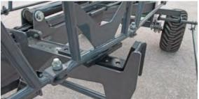
For road transport, the rotors are placed on the frame. This protects the pivot joints, as there is no stress on them at all when they are folded in. The special transport position, with the rotors lined up in a row, means that even the larger Lotus models are compact enough for transport.
