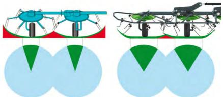
The Fendt Performance tines act in a dragging motion – but with their hook solution and high flexibility, they glide across the ground without damaging the sward. They have a very large pickup range compared to conventional tines, giving you greater area coverage.
