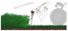
The extra stable tine arms are designed for high power transmission and maximum durability.
