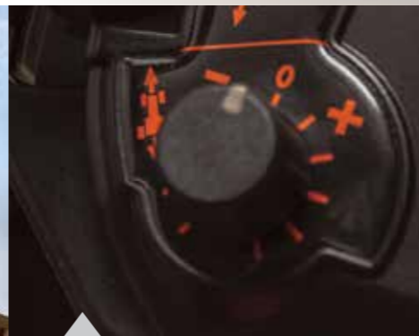
Comfort Control roller switch PowerControl lever option : Shuttle responsiveness can be adjusted according to speed of change required to really match the handling job in hand
